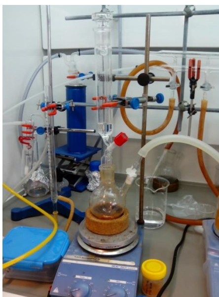
Fig. 8. System at reduce pressure during the addition of benzyl alcohol.
