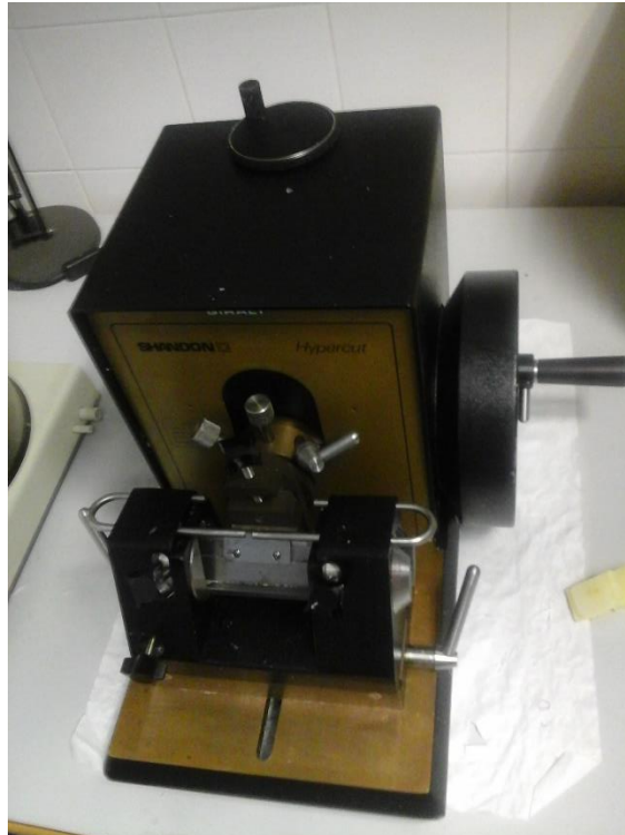
Figure 16: The microtome (Hypercut).
