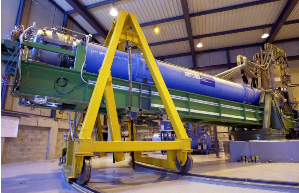
Figure 2.1: Experimental set-up of the CAST experiment. The dipole magnet (blue) is mounted on a movable platform (green) that allows the horizontal and vertical movement.
