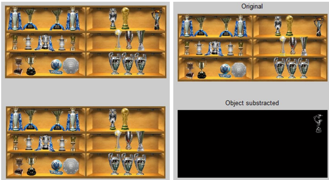
Figure 4.2: On the left side can be seen the original image, and below the current image, with the trophy missing. On the other hand, on the right side can be seen how Kyle's glasses detected the trophy that was missing, on the corner of the glass cabinet.
