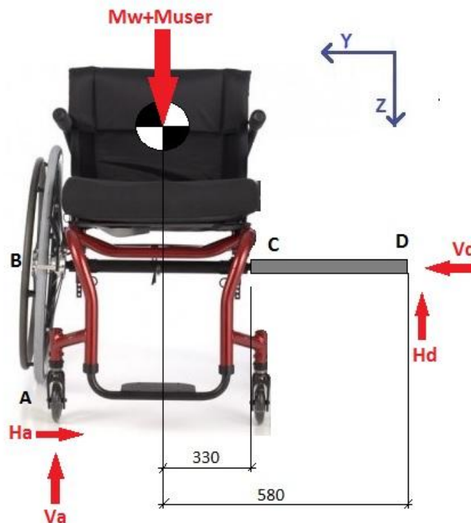
Figure 8.7. Free body diagram of a static simulation on the wheelchair with the first bar attached to the quick release.
