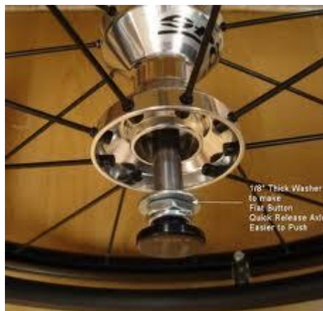
Figure 8.8. Quick release briefly extracted from its bushing.
