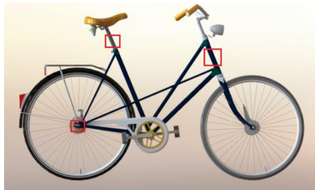
Figure 8.4. Attachment point locations on a urban bicycle.
