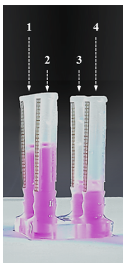
Fig. 2.6. Application of pressure gradient. It is employed for measuring the permeability of the scaffold hydrogels.
