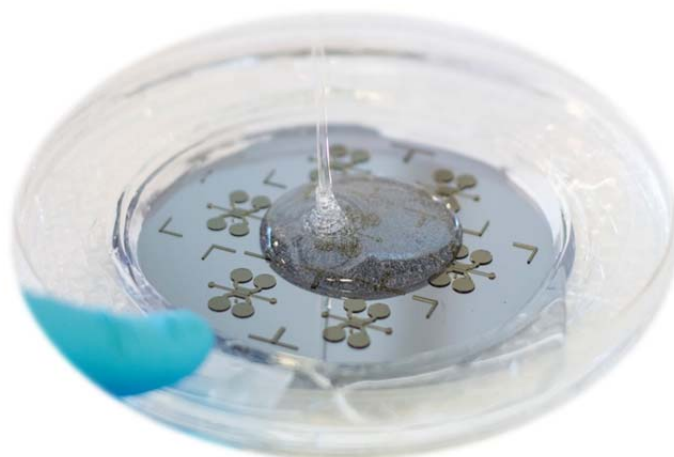
Fig. 2.3. PDMS pouring. The liquid polymer is spilled onto the SU8 mold in order to let it cast patterned, after degassing it.
