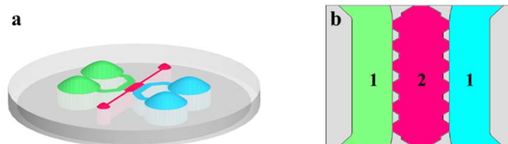
Fig. 4.1. Geometry of the microfluidic device. A general view of the microdevice is shown in picture (a). The central area is demonstrated as a top view in picture (b), in which the geometry and nomenclature of the compartments are detailed: the channel (1) and the hydrogel (2) compartments. The hydrogel is injected into the central cavity (pink), whose dimensions are 2.5 x 1.3 mm; the main channels (green and blue) are filled with culture media or PBS. When a GF or dextran is added in order to establish a chemical gradient, it is included in the addition channel (green) and diffuses through the hydrogel towards the opposite channel (blue).
