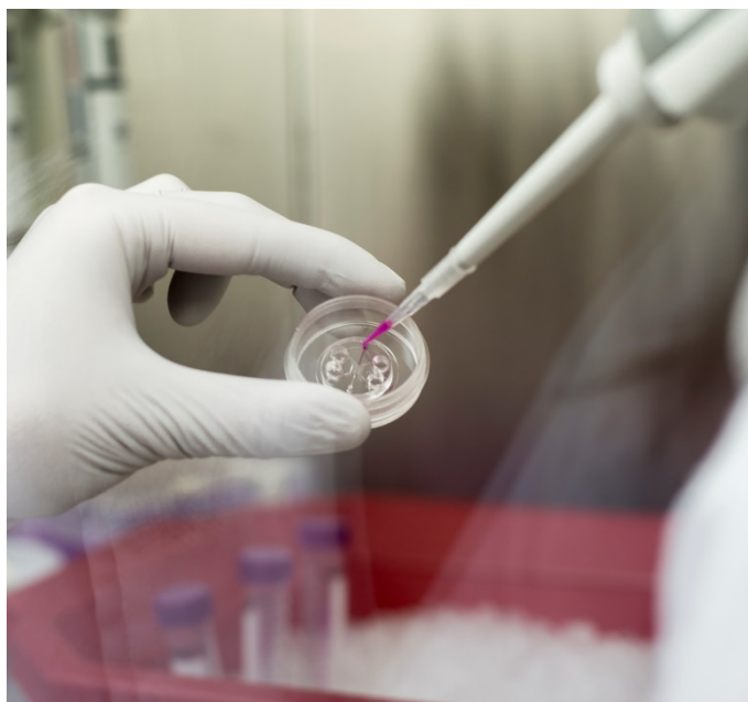
Fig. 2.4. Hydrogel injection. Once the gel solution is readily mixed and placed on ice, the necessary amount is pipetted into the microfluidic device.
