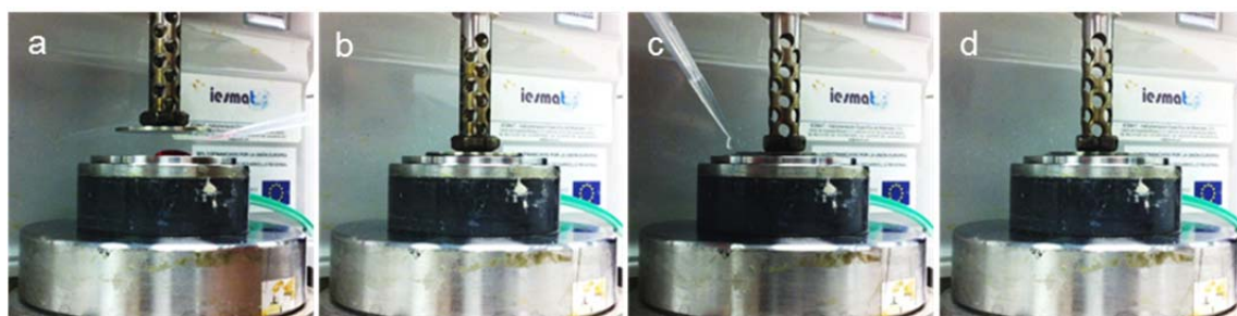
Fig. 3.2. Sequenced pictures of the gel filling process on the rheometer. Once the sample was mixed, it was pipetted on the rheometer plate (a), adjusted the gap (b), covered with the oil (c) and got ready to run the experiment (d).
