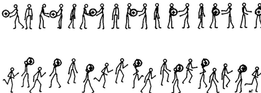
Fig. 6.10 Models for proton conduction via (a) Grotthuss Mechanism (protons jump from one molecule to a neighboring one within an extended hydrogen-bond net) and (b) Vehicle Mechanism (a vehicle molecule or carrier assists the movement, and the proton is transferred as a complex ion). Reproduced from Kreuer et al. 1982. [60]
