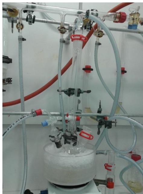
Figure 18. 2-neck flask placed under dynamic vacuum and at 0°C
