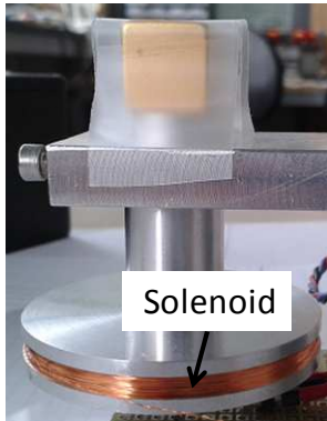
Figure 16: The coil used to vary the position of the magnet levitated.
