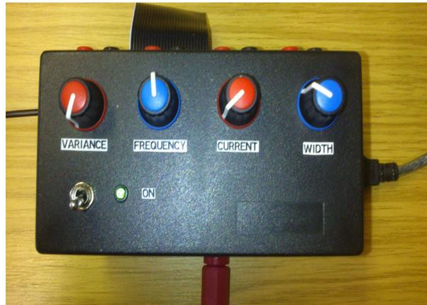
Fig 5. Stimberry controller. Front potentiometers
