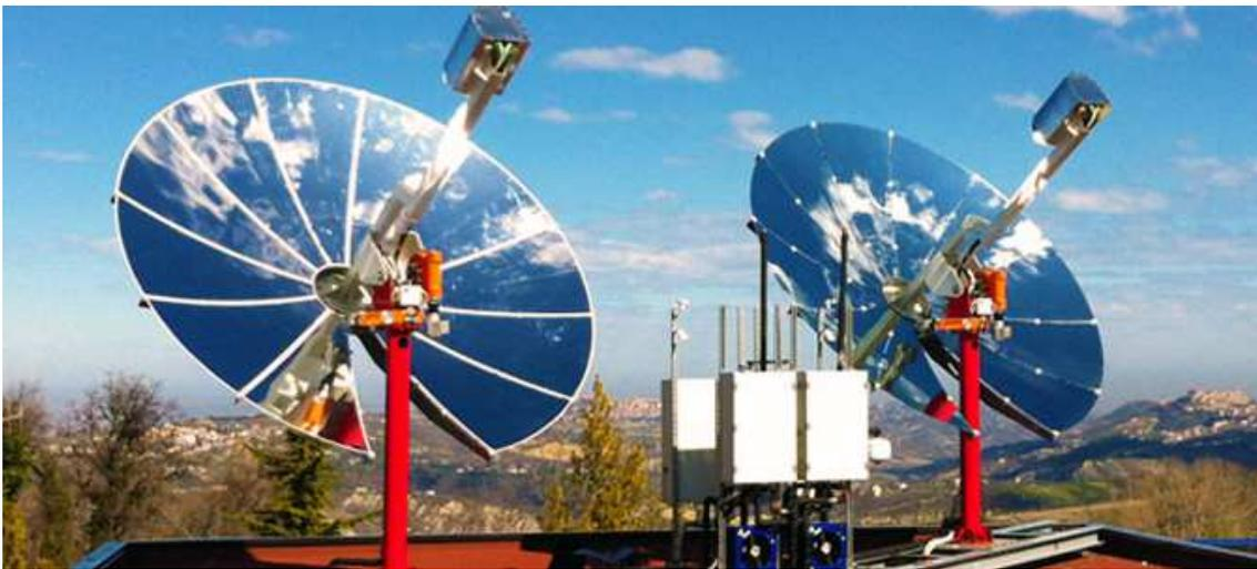
Figura 22 Sistema disco-Stirling Innova [33].
