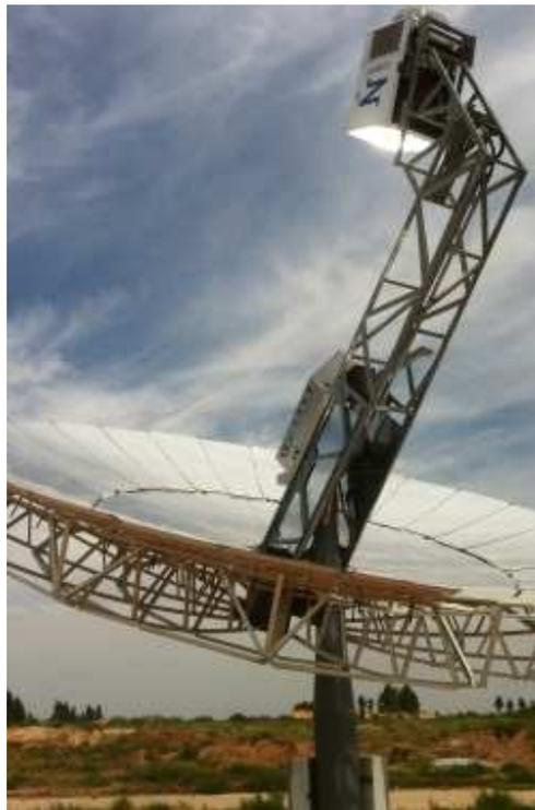
Figura 20 Sistema disco-Stirling Cleanergy [30].
