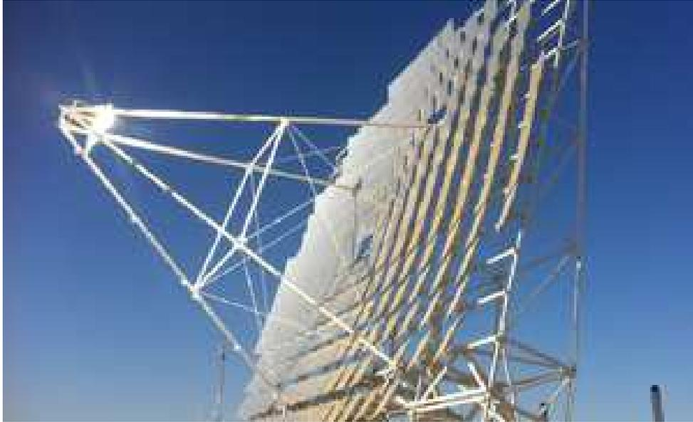
Figura 23 Sistema disco-Stirling HelioFocus [34].
