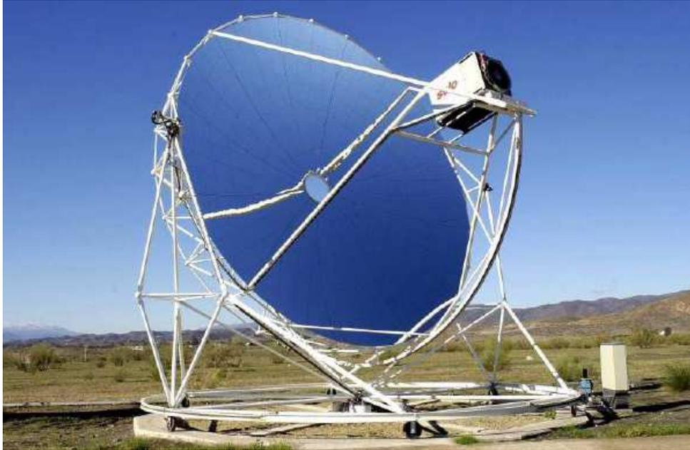
Figura 24 Sistema disco-Stirling SBP [25].
