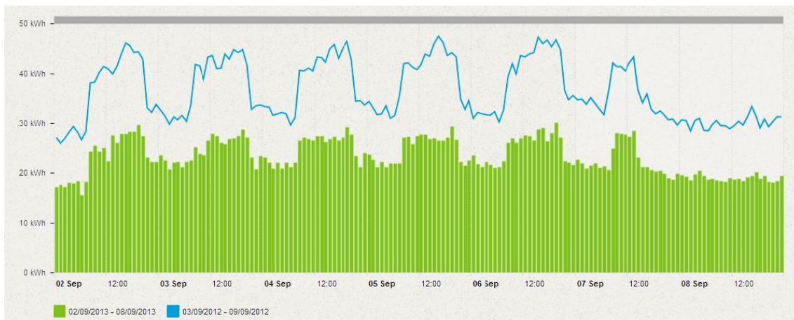
Figure 9. Consumption of energy related with the vertical refrigerated shelves (ANESE. Casos de éxito: Caso de estudio Berriak)
