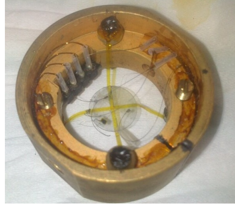
Fig.14: Isoperibol calorimeter brought from Kamerlingh Onnes Laboratorium of the University of Leiden, used as example in the development of our own. Some parts have been used in our model.
