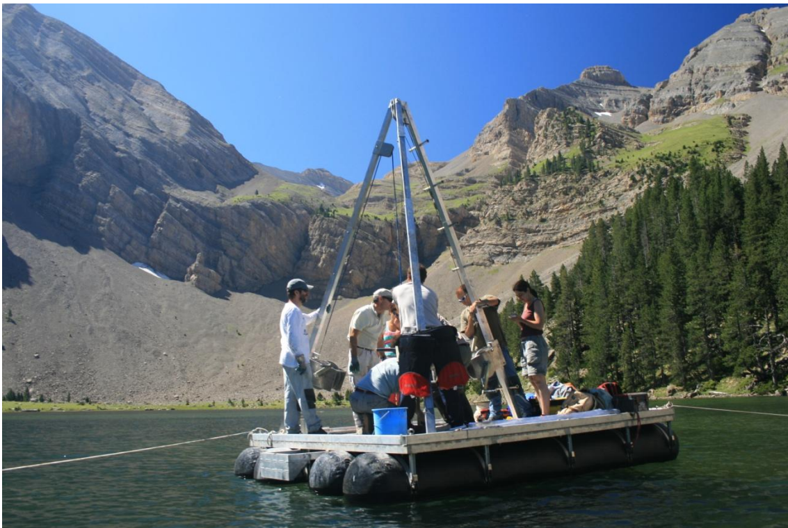
Figure 2.7. Core drilling campaign in Lake Basa de la Mora (2008).
