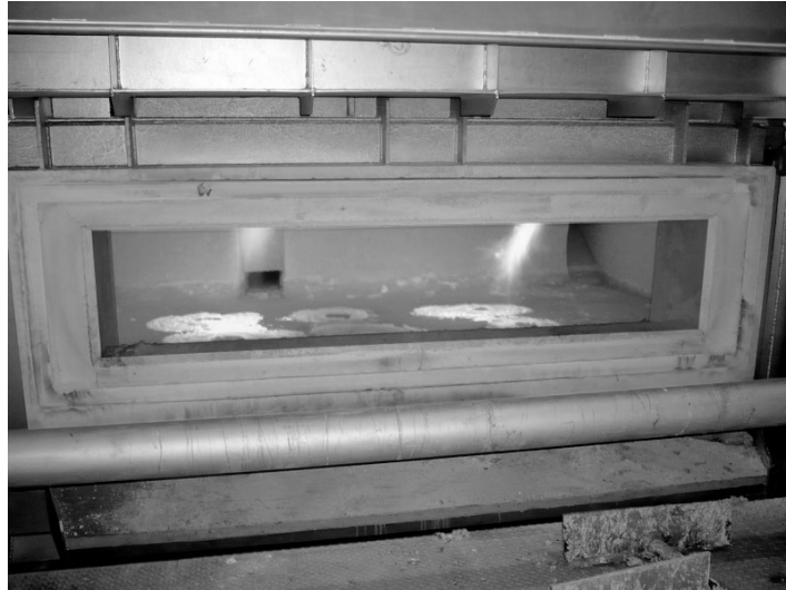
Figure 2.24. Reverberatory furnace heated by direct combustion flame (StrikoMelter, 2013)
