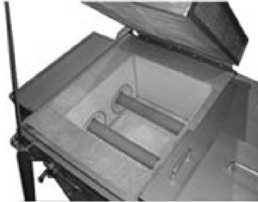
Figure 2.27. Electric immersion holding furnace (SPX, 2013)
