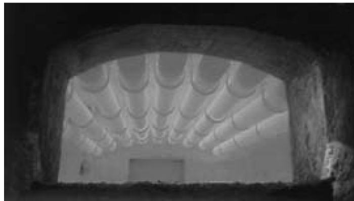
Figure 2.25. Radiant tube in reverberatory furnace (Khanthal, 2011)
