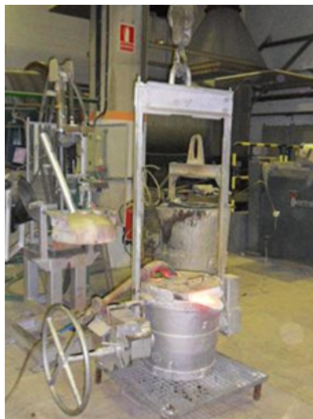
Figure 4.4. Preheating process for the ladle with a gas burner
