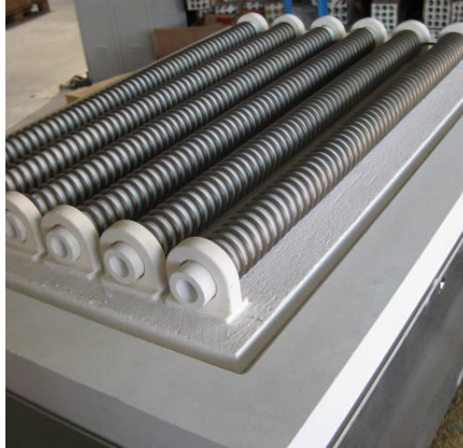
Figure 5.2. Photograph of the electrical resistances array
