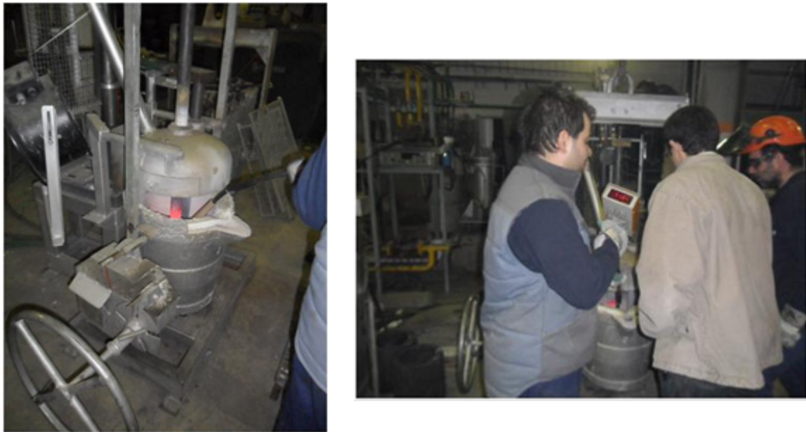
Figure 4.7. Measurement of molten temperature
