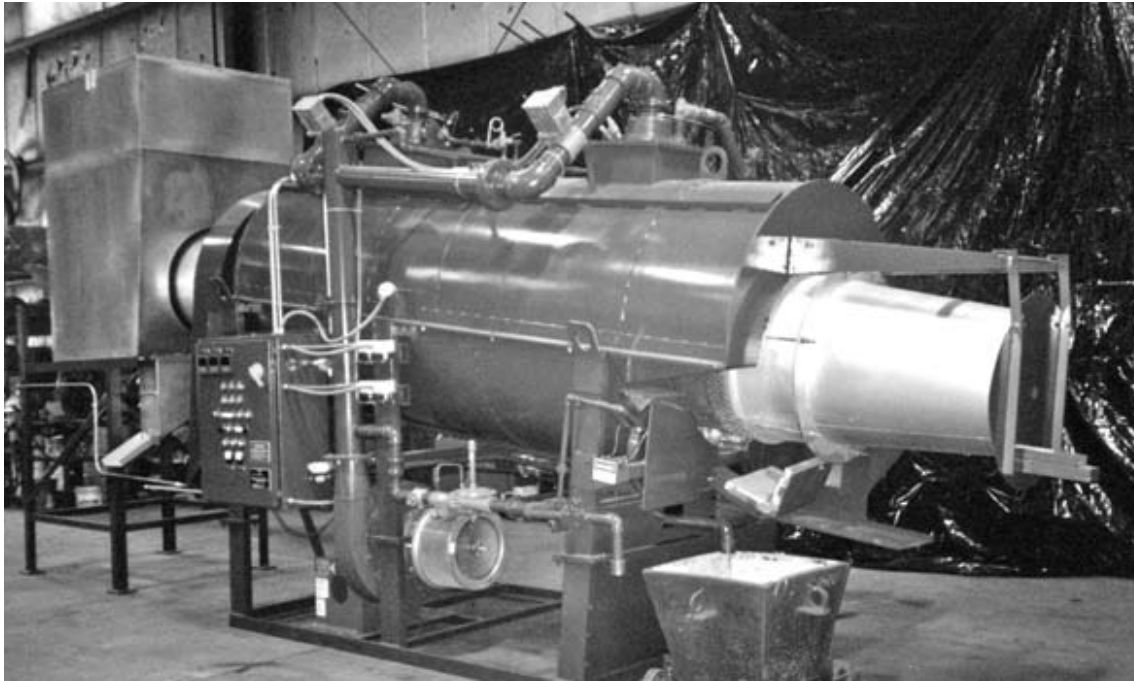
Figure 2.12. Large-scale rotary sweat furnace (Schlesinger, 2006)
