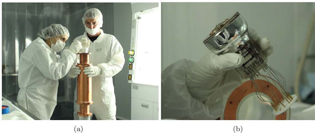
Figure 6.2: PMT coupling to the ANAIS-25 modules in the LSC clean room: (a) connecting the PMT flying leads into the voltage divider connectors, and (b) PMT with the optical grease on it, just before coupling it to the quartz window.
