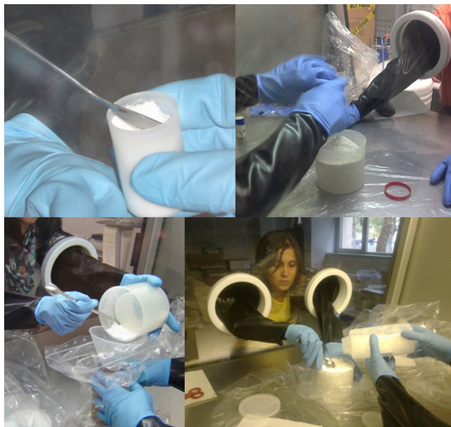
Figure 5.2: Pictures of the preparation of different NaI samples at the glove box, at the University of Zaragoza.
