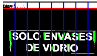
Figure 8. Final evaluation of segments in the hypothesis area. Long segments still found inside the region (top segment, in red) are used to crop it. Distribution of small segments (in green) inside the 8 region cells (marked with long vertical edges) is used to update the hypothesis likelihood of containing text.
