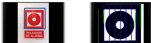
Figure 10. Re-evaluation step provides better likelihood estimation in cases where simple histogram analysis fails. This example got high P_{ini} but low P_{lines} , properly decreasing the final likelihood of being text because there are very few straight segments (green).
