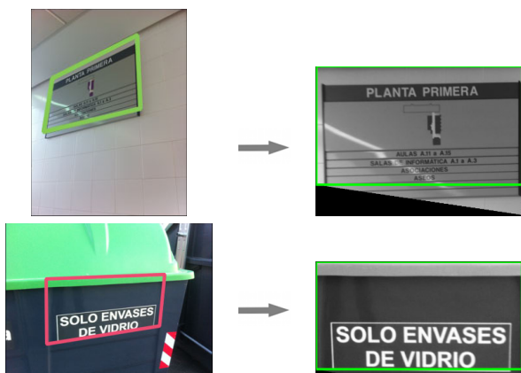
Figure 7. Two examples of the projection from an original image (left) to a virtual frontal view (right).
