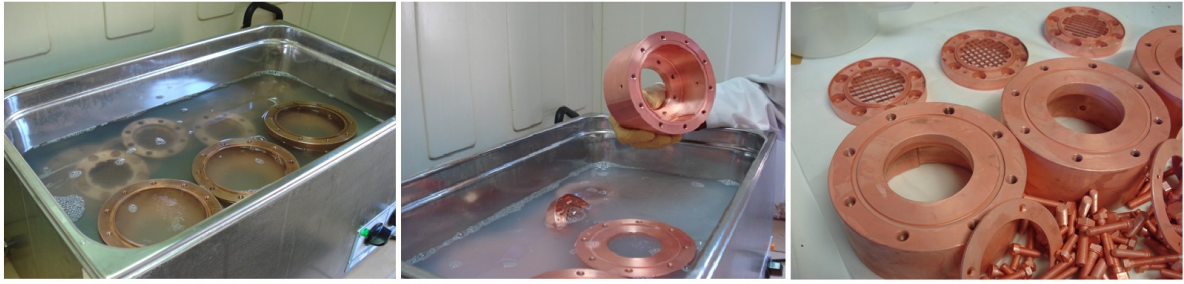
Figure 14. Cleaning process. Soap Cleaning and Acid Etching.
