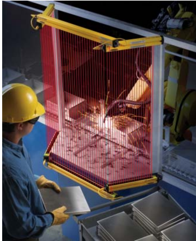
Illustration 1: Infrared curtain in a factory.
