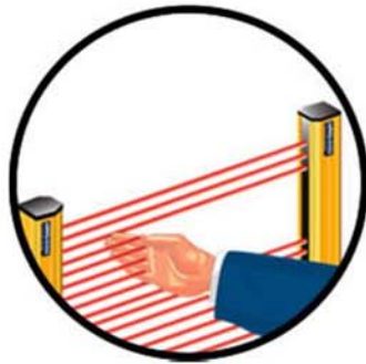
Fig 1.a: Infrared Light Curtain (Light Curtain and Machine Guard Solutions, 2009)
