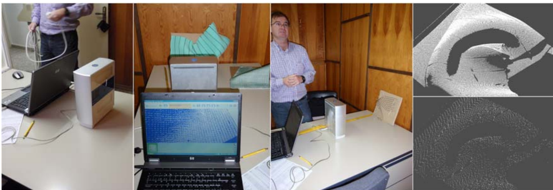
Figure 2.6: Laser scan digitalization with a very high-resolution scanner. It gives extremely dense point-clouds of the scanned surface. The use of only one scanner source impedes the total reconstructions of the complex model (shadows in figure).
