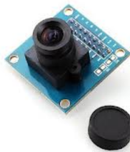
Fig.2: OV7670 Digital Image Sensor with Optical Lens.
