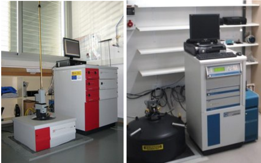
Figure 7: MPMS (left) and PPMS (right) used in the samples characterization.
