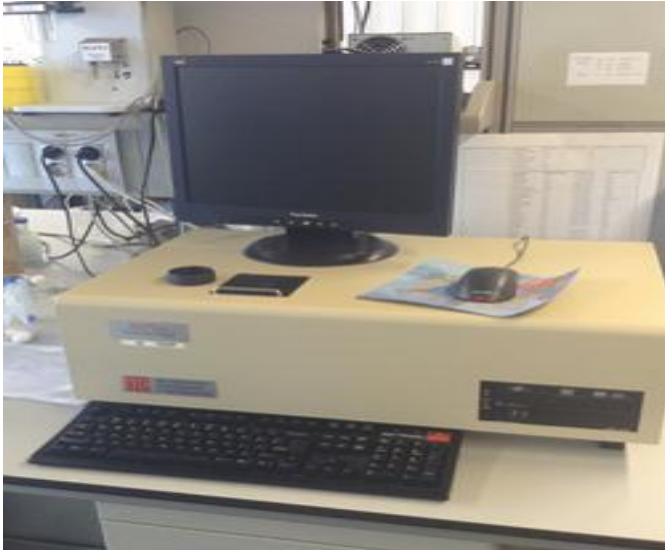
Brookhaven 90 plus photo correlation spectroscopy used for particle size analysis (DLS)
