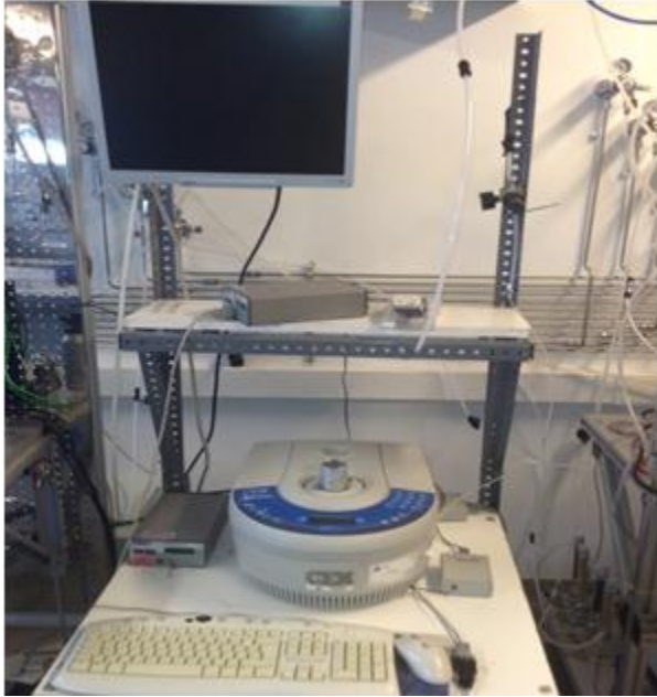
CEM microwave system used to synthesize silver nano spheres.
