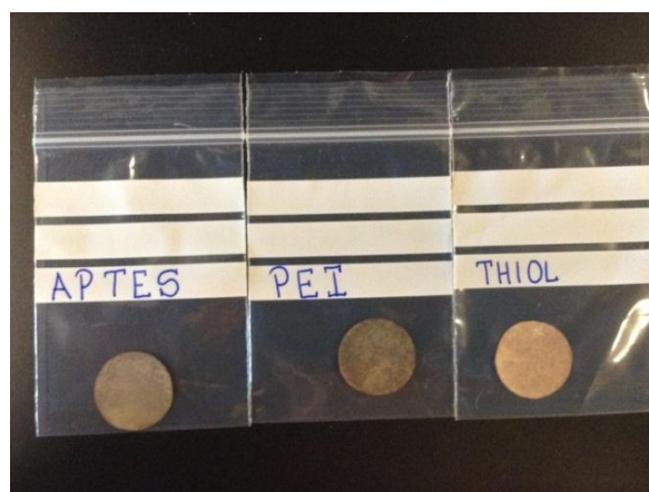
Figure 24 The photo images of a) APTES b) PEI and c) Thiol -modified cellulose filter after the attachment of Ag NPs.
