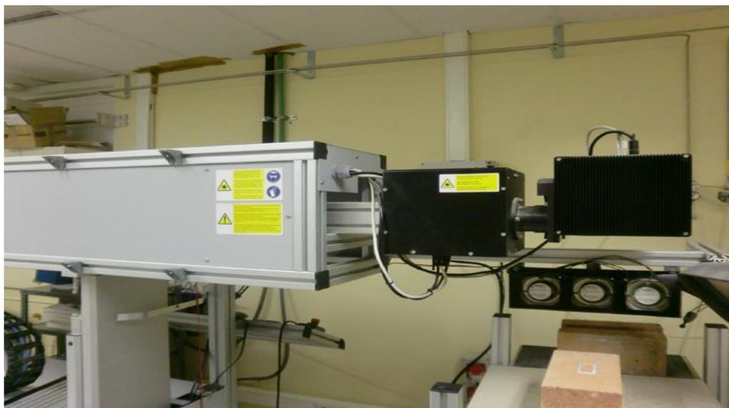
*Figura 11 .Laser Rofin-Sinar SLAB CO<sub>2</sub>.*
