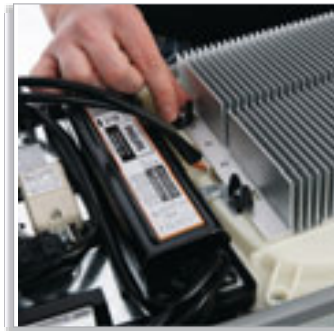
Easy re-LEDing without use of tools (unlocking the LED module)
