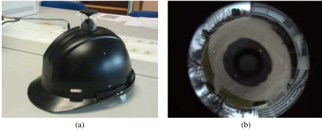
Figure 1.1: (a) Hemlet-camera device used in our experiments. (b) Omnidirectional image captured with our device.
