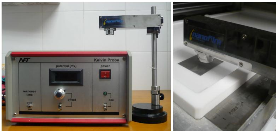
Figure 3.3. Kelvin Probe SP1 instrument provided by Nanofilm for surface potential vs. area per molecule measurements [47].
