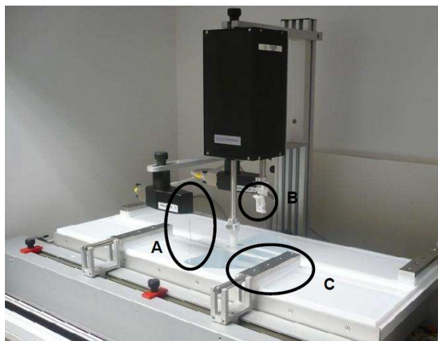
Figure 2.1. KSV Commercial Langmuir trough. A) Wilhelmy balance. B) Dipper. C) Mobile barriers [47].
