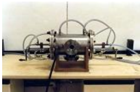
Figure 6: Arc discharge reactor used for the synthesis of SWNTs.
