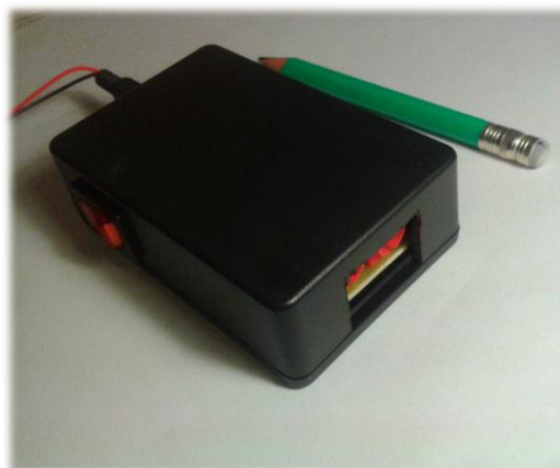
Figure 6.2: Complete vibration sensor module.
