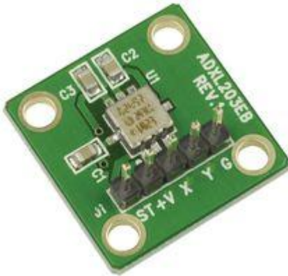
Figure 3.5: ADXL Evaluation board
