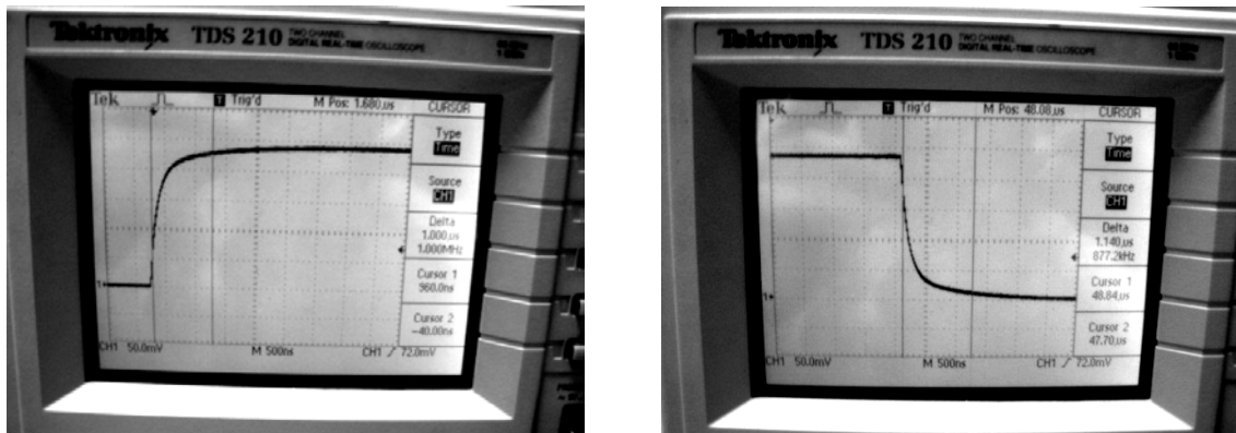
(a) (b) Fig.52: (a) Blue LED 3 mm rise time. (b) Blue LED 3 mm fall time.
