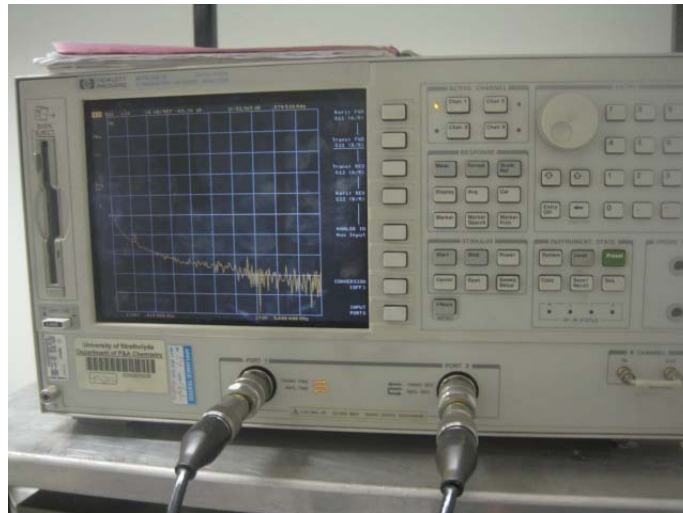
Fig.63: S-parameter analyzer used during the experiment.
