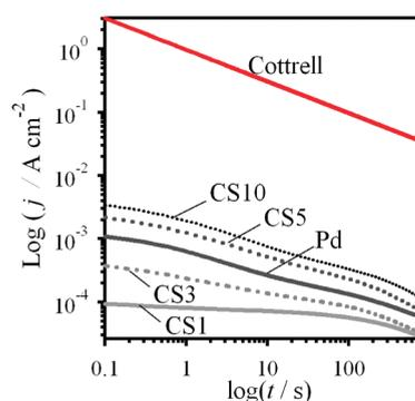
**Figure 8.** Log–log representation of chronoamperometric transients for HCOOH oxidation on Pd and CS nanoparticle assemblies, at  $0.4 \text{ V}$  in  $0.5 \text{ mol dm}^{-3} \text{ H}_2\text{SO}_4$  and  $2 \text{ mol dm}^{-3} \text{ HCOOH}$ . In all cases, it can be seen that the current responses are orders of magnitude lower than the Cottrell (diffusional) limit.
