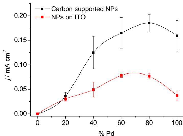
**Figure 4.31.** Current density at 750 seconds associated with HCOOH oxidation at 0.60 V (vs. RHE), on the various metallic nanostructures assembled on ITO (red) and supported on Vulcan (black), in 0.5 M H<sub>2</sub>SO<sub>4</sub> + 2 M HCOOH.
