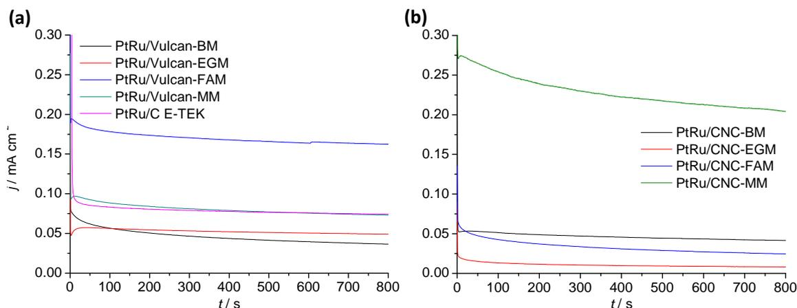
**Figure 4.17.** Chronoamperometric curves for the PtRu/Vulcan (a) and PtRu/CNC (b) electrocatalysts, recorded in 2 M  $\text{CH}_3\text{OH}$  + 0.5 M  $\text{H}_2\text{SO}_4$  solution, at  $E = 0.60$  V and room temperature.
