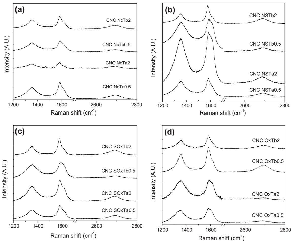
**Fig. 2.** Raman patterns obtained for: (a) Samples treated with  $\text{HNO}_3$ ; (b) Samples treated with  $\text{HNO}_3\text{--H}_2\text{SO}_4$ ; (c) Samples treated with  $\text{H}_2\text{SO}_4\text{--H}_2\text{O}_2$ ; and (d) Samples treated with  $\text{H}_2\text{O}_2$ .
