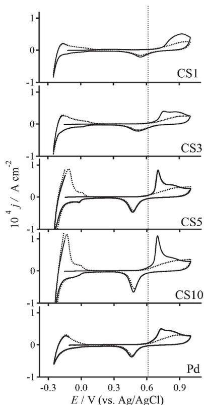
**Figure 5.** CO stripping voltammograms at  $20 \text{ mV s}^{-1}$  of the various core–shell and Pd nanoparticle assemblies. Potential scans were initiated at open circuit potential. The dotted voltammograms show the second scan after CO desorption. The vertical dotted line corresponds to the onset of CO oxidation at Pd nanoparticles. The composition of the assembly and electrolyte solution are indicated in the caption of Figure 4.
