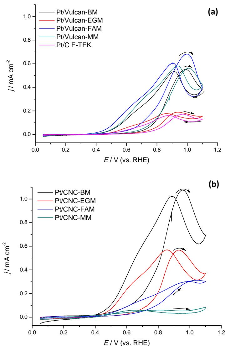
**Figure 4.20.** Cyclic voltammograms for Pt/Vulcan (a) and Pt/CNC (b) electrocatalysts in 2M  $\text{CH}_3\text{CH}_2\text{OH} + 0.5\text{M H}_2\text{SO}_4$ .  $v = 0.02 \text{ V s}^{-1}$ ;  $T = 25 \text{ }^\circ\text{C}$ .
