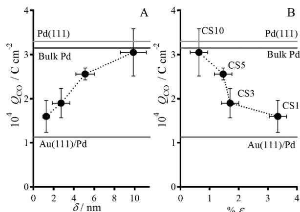
**Figure 6.** Average charge density of CO oxidation ( $Q_{\text{CO}}$ ) as a function of Pd thickness,  $\delta$ , (A), and lattice strain,  $\epsilon$ , (B) in Au–Pd core–shell nanostructures. The characteristic charges for bulk Pd(111),<sup>7</sup> polycrystalline,<sup>48</sup> and pseudomorphic monolayer on Au(111) surfaces<sup>6</sup> are indicated.
