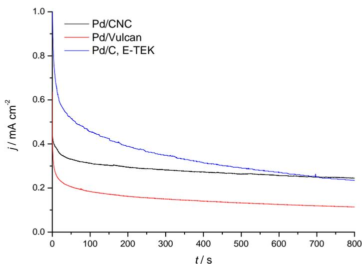
**Figure 4.19.** Chronoamperometric curves for the Pd based electrocatalysts, recorded in 2 M HCOOH + 0.5 M H<sub>2</sub>SO<sub>4</sub> solution, at E = 0.60 V and room temperature.
