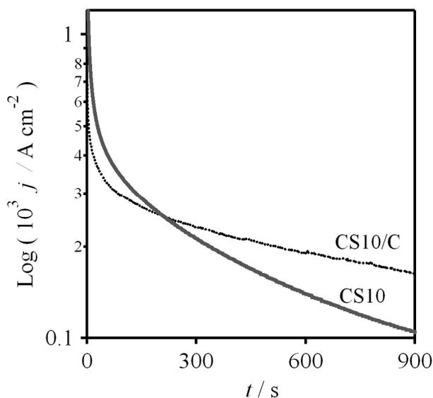
**Figure 7.** Comparison of transients associated with HCOOH oxidation on CS10 nanoparticles assembled at ITO (CS10/ITO) and supported on Vulcan (CS10/C), at 0.40 V. The composition of the electrolyte solution can be found in the caption of **figure 6**.
