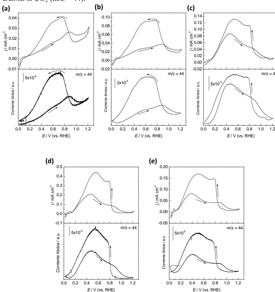
**Figure 4.32.** DEMS experiments for the electrodes: CS1/C (a), CS3/C (b), CS5/C (c), CS10/C (d) and Pd/C (e); in 0.5 M HCOOH + 0.5 M H<sup>2</sup>SO<sub>4</sub>,  $v = 0.001 \text{ V s}^{-1}$ ;  $T = 25 \text{ }^\circ\text{C}$ .
