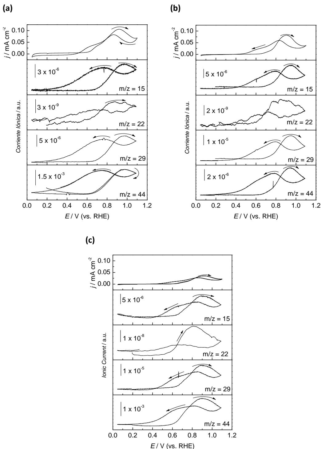
**Figure 4.22.** CVs and MSCVs for 0.5 M ethanol oxidation in 0.5 M H<sub>2</sub>SO<sub>4</sub>, at Pt/CNC-BM (a), Pt/Vulcan-FAM (b) and Pt/C E-TEK (c).  $v = 0.001 \text{ V s}^{-1}$ ;  $T = 25 \text{ }^\circ\text{C}$ .
