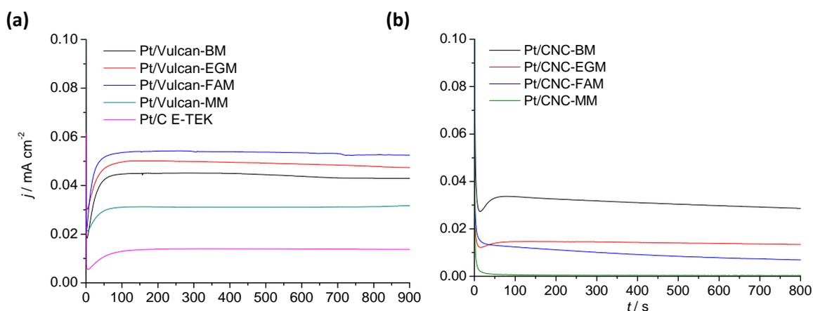
**Figure 4.16.** Chronoamperometric curves for the Pt/Vulcan (a) and Pt/CNC (b) electrocatalysts, recorded in 2 M CH<sub>3</sub>OH + 0.5 M H<sub>2</sub>SO<sub>4</sub> solution, at  $E = 0.60$  V and room temperature.
