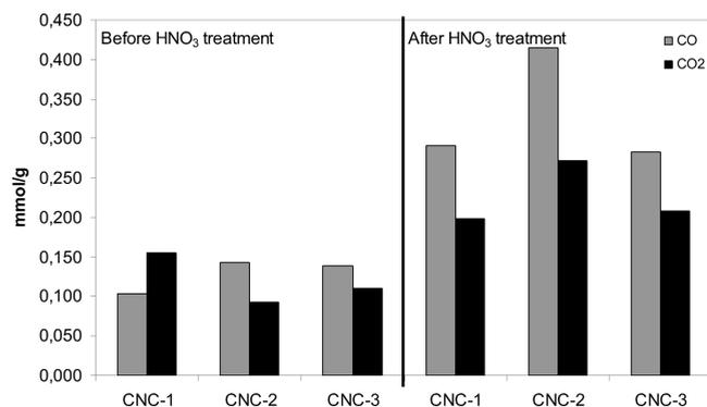
**Figure 6.** Total CO and CO<sub>2</sub> amount desorbed during the TPD experiments carried out before and after the HNO<sub>3</sub> treatment.
