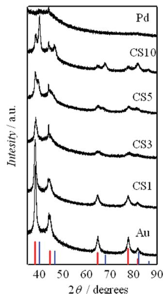
**Figure 2.** Powder XRD diffractograms of Au, Pd, CS1, CS3, CS5, and CS10 nanoparticles. The red lines at  $38.1^\circ$ ,  $44.4^\circ$ ,  $64.6^\circ$ ,  $77.5^\circ$ , and  $81.7^\circ$  indicate the standard Au diffraction pattern, while the blue lines at  $40.1^\circ$  (111),  $46.7^\circ$  (200),  $68.1^\circ$  (220),  $82.1^\circ$  (311), and  $86.6^\circ$  belong to Pd.
