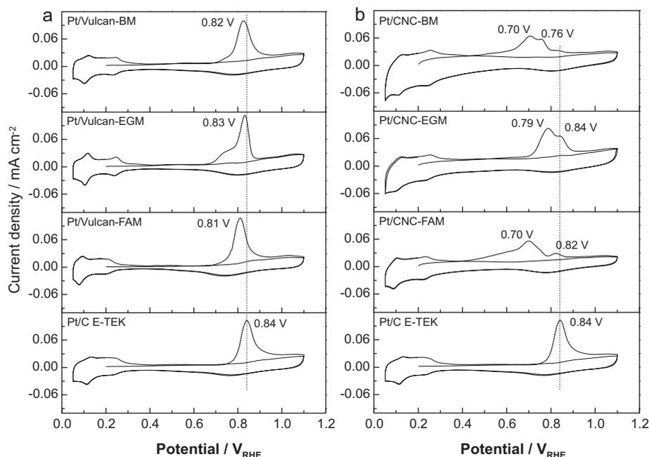
**Fig. 2.** CO-stripping voltammeteries for Pt/Vulcan (a) and Pt/CNC (b) electrocatalysts in 0.5 M H<sub>2</sub>SO<sub>4</sub>,  $E_{ad} = 0.20$  V;  $\nu = 20$  mV s<sup>-1</sup>;  $T = 25$  °C.
