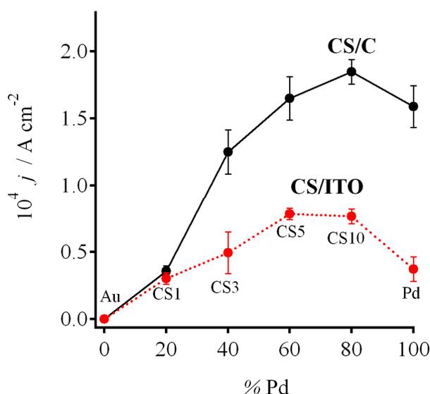
**Figure 8.** Current density at 750 seconds associated with HCOOH oxidation at 0.40 V on the various metallic nanostructures assembled on ITO (red) and supported on Vulcan (black). See caption of **figure 6** for the composition of the electrolyte solution.
