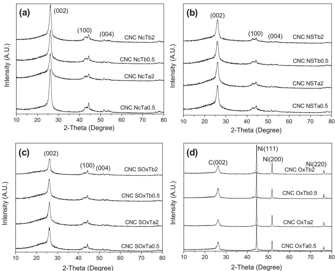
**Fig. 1.** XRD patterns obtained for: (a) Samples treated with  $\text{HNO}_3$ ; (b) Samples treated with  $\text{HNO}_3\text{--H}_2\text{SO}_4$ ; (c) Samples treated with  $\text{H}_2\text{SO}_4\text{--H}_2\text{O}_2$ ; and (d) Samples treated with  $\text{H}_2\text{O}_2$ .
