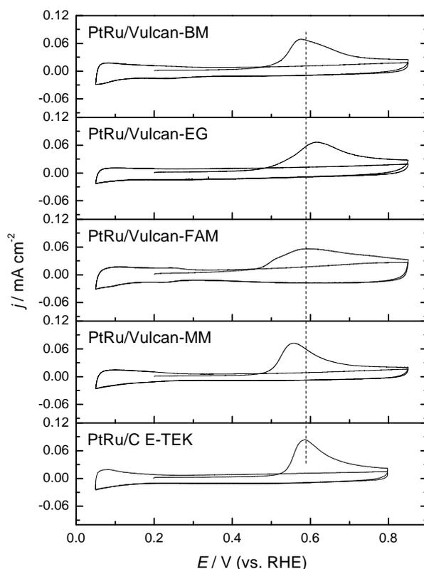
**Figure 4.11.** CO-stripping voltammograms for the PtRu/Vulcan electrocatalysts in 0.5 M  $\text{H}_2\text{SO}_4$ .  $E_{\text{ad}} = 0.20$  V;  $v = 0.020$  V  $\text{s}^{-1}$ ;  $T = 25$  °C.
