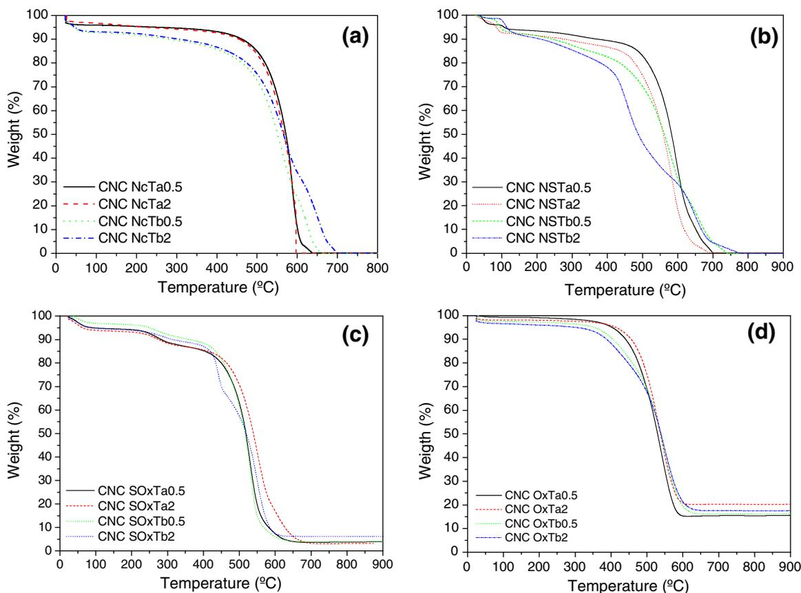
**Fig. 3.** Thermogravimetric weight change curves under air atmosphere for: (a) Samples treated with  $\text{HNO}_3$ ; (b) Samples treated with  $\text{HNO}_3\text{-H}_2\text{SO}_4$ ; (c) Samples treated with  $\text{H}_2\text{SO}_4\text{-H}_2\text{O}_2$ ; and (d) Samples treated with  $\text{H}_2\text{O}_2$ .
