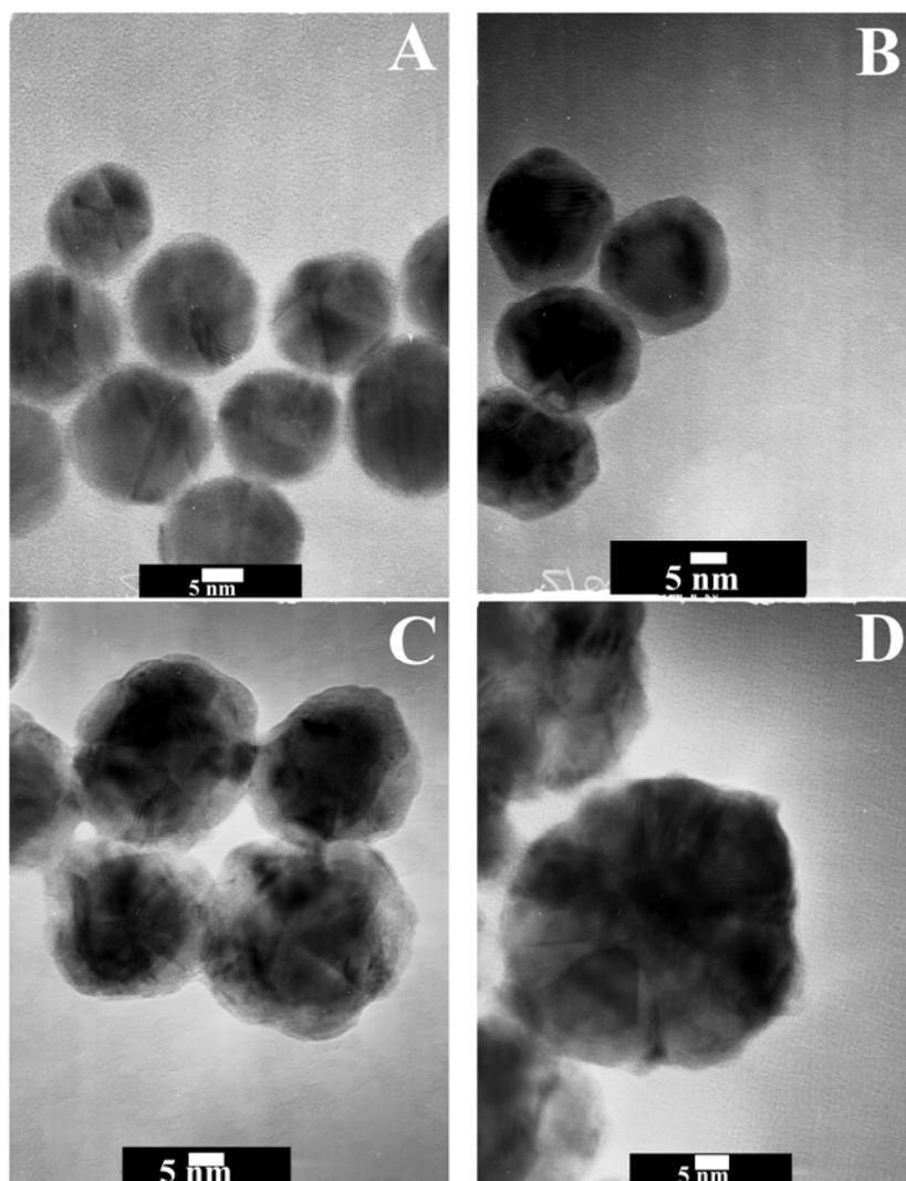
**Figure 4.25.** HRTEM images of the core-shell nanoparticles featuring  $19.3 \pm 1.2$  nm Au cores, coated with Pd shells with thickness of  $1.3 \pm 0.09$  nm (A),  $2.7 \pm 0.1$  nm (B),  $5.1 \pm 0.9$  nm (C) and  $9.9 \pm 1.0$  nm (D) [MONTES DE OCA 2012].
