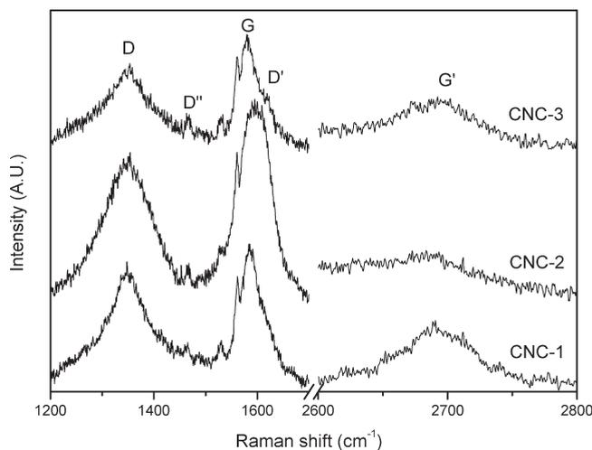
Figure 2. First- and second-order Raman spectra of CNCs.
