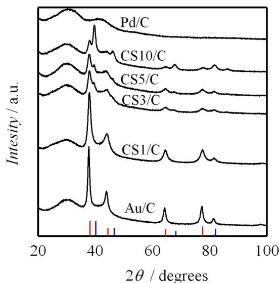
**Figure 3.** Powder XRD diffractograms of the various metallic nanostructures supported on Vulcan support. Composition and dimension of the various samples are indicated in **table 1**.
