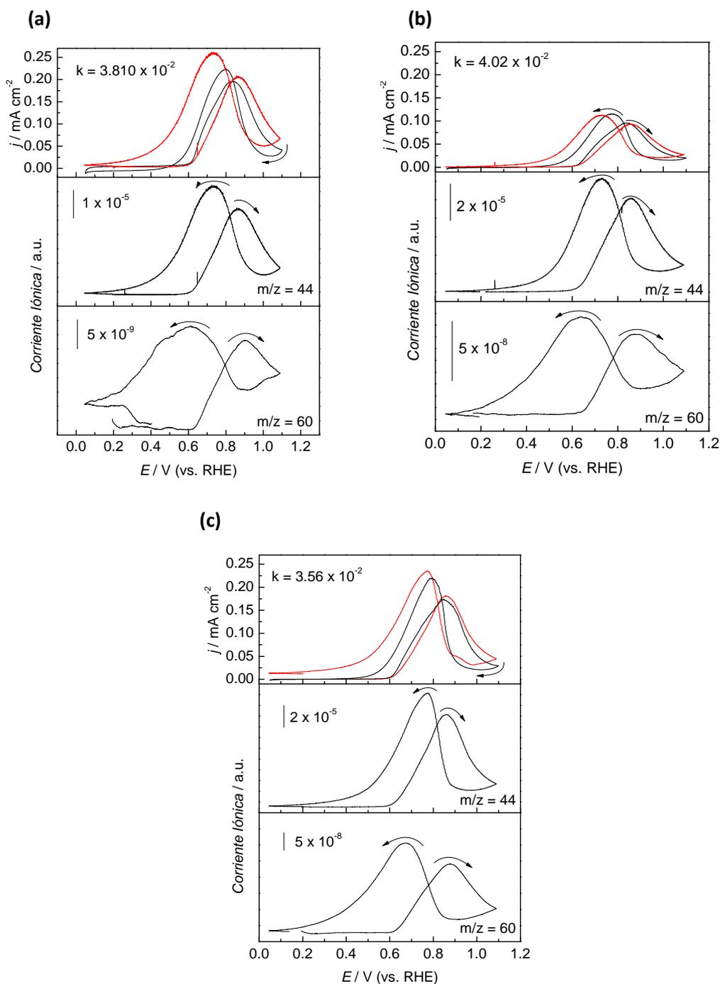
**Figure 4.18.** CVs and MSCVs for 0.5 M methanol oxidation in 0.5 M  $\text{H}_2\text{SO}_4$  at Pt/CNC-BM (a), Pt/Vulcan-FAM (b) and Pt/C E-TEK (c).  $v = 0.001 \text{ V s}^{-1}$ ;  $T = 25 \text{ }^\circ\text{C}$ .
