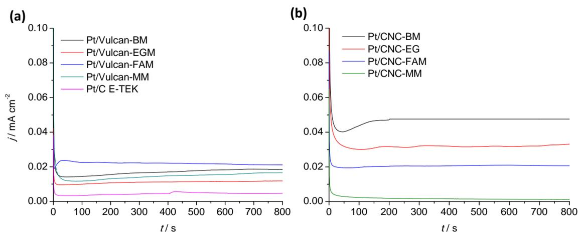
**Figure 4.21.** Chronoamperometric curves for Pt/Vulcan (a) and Pt/CNC (b) electrocatalysts, recorded in 2 M  $\text{CH}_3\text{CH}_2\text{OH}$  + 0.5 M  $\text{H}_2\text{SO}_4$  solution, at  $E = 0.60$  V and room temperature.
