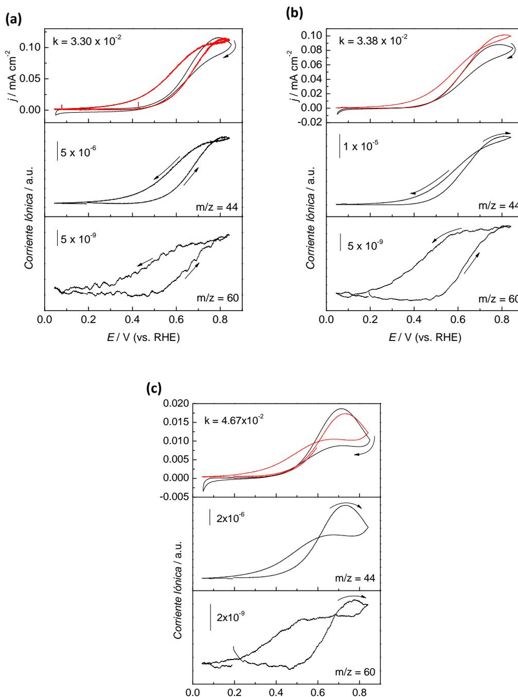
**Figure 4.19.** CVs and MSCVs for 0.5 M methanol oxidation in 0.5 M  $\text{H}_2\text{SO}_4$  at PtRu/CNC-MM (a), PtRu/Vulcan-FAM (b) and PtRu/C E-TEK (c).  $v = 0.001 \text{ V s}^{-1}$ ;  $T = 25 \text{ }^\circ\text{C}$ .
