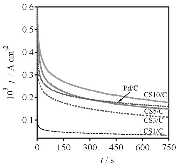
**Figure 6.** Chronoamperometric transients of Pd and CS catalysts supported on Vulcan at 0.40 V, in 2 mol dm<sup>-3</sup> HCOOH and 0.5 mol dm<sup>-3</sup> H<sub>2</sub>SO<sub>4</sub>.
