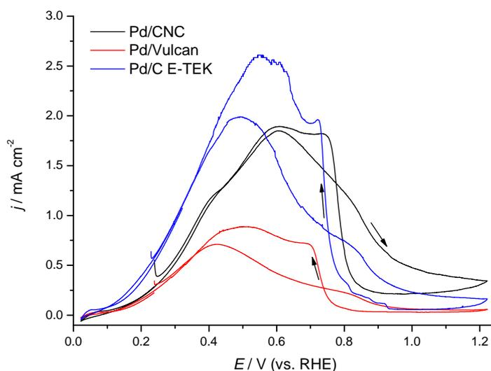
**Figure 4.23.** Cyclic voltammograms for Pd/CNC, Pd/Vulcan and Pd/C from E-TEK electrocatalysts recorded in  $2 \text{ M HCOOH} + 0.5 \text{ M H}_2\text{SO}_4$ .  $v = 0.020 \text{ V s}^{-1}$ ;  $T = 25 \text{ }^\circ\text{C}$ .
