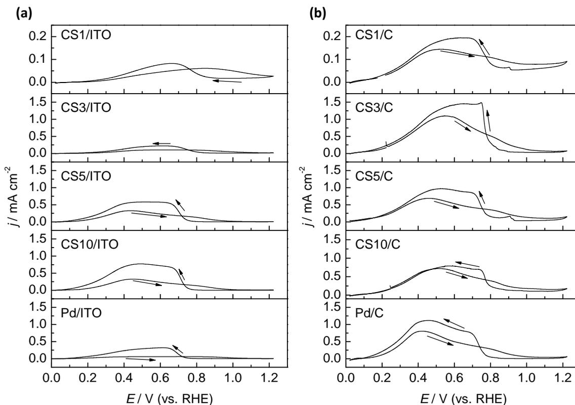
**Figure 4.30.** Cyclic voltammograms of the core-shell and Pd nanoparticles assembled on ITO (a) and supported on Vulcan (b), at  $0.02 \text{ V s}^{-1}$ , in 2 M HCOOH + 0.5 M H<sub>2</sub>SO<sub>4</sub>.
