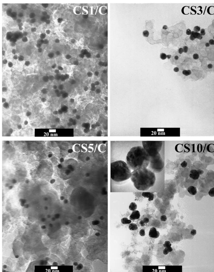
**Figure 4.26.** TEM images of the various CS nanoparticles supported on Vulcan. The inset in CS10 is an image with higher magnification, showing the contrast between the Au core and the Pd shell [CELORRIO 2012].
