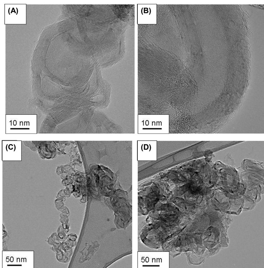
**Figure 4.4.** HRTEM (A and B) and TEM (C and D) images of CNC-3.
