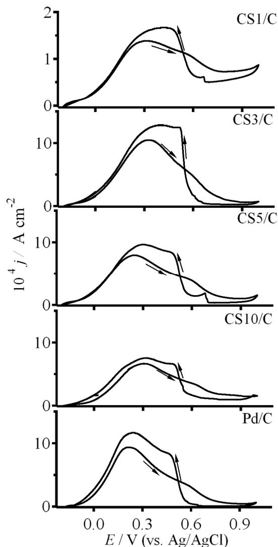
**Figure 5.** Cyclic voltammograms of the various nanostructures supported on Vulcan in the presence of  $2 \text{ mol dm}^{-3} \text{ HCOOH}$  and  $0.5 \text{ mol dm}^{-3} \text{ H}_2\text{SO}_4$ , at  $0.02 \text{ V s}^{-1}$ .
