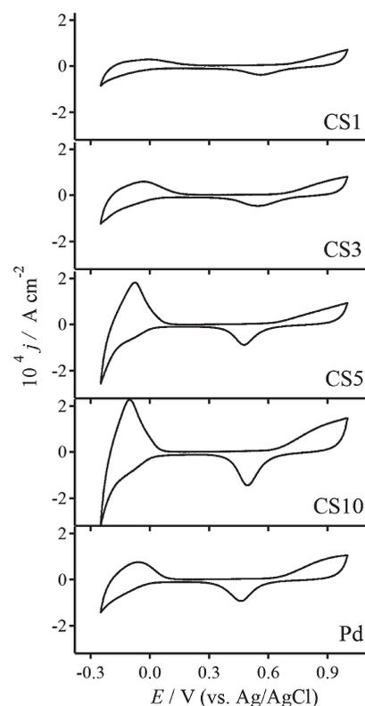
**Figure 4.** Cyclic voltammograms at  $100\ \text{mV s}^{-1}$  of  $5 \times (\text{CS}:\text{PLL})$  assemblies featuring CS1, CS3, CS5, and CS10. These responses are compared with the voltammogram of a  $5 \times (\text{Pd}:\text{PLL})$  assembly (Pd). The electrolyte solution was  $0.5\ \text{mol dm}^{-3}\ \text{H}_2\text{SO}_4$ .
