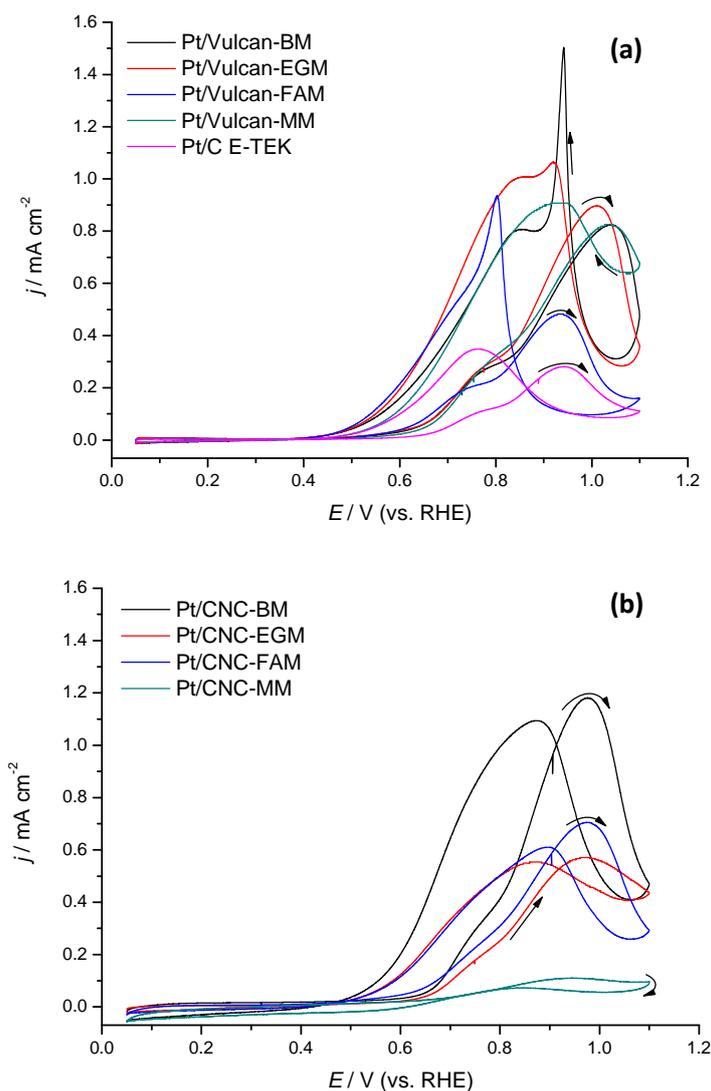
**Figure 4.14.** Cyclic voltammograms for Pt/Vulcan (a) and Pt/CNC (b) electrocatalysts in 2 M CH<sub>3</sub>OH + 0.5 M H<sub>2</sub>SO<sub>4</sub>,  $v = 0.02 \text{ V s}^{-1}$ ;  $T = 25 \text{ }^\circ\text{C}$ .
