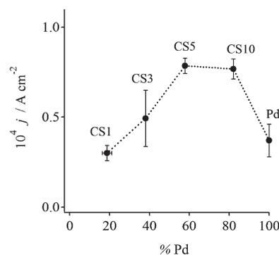
**Figure 9.** Current densities of HCOOH oxidation after  $750 \text{ s}$  at  $0.4 \text{ V}$  at the nanoparticle assemblies expressed in terms of the Pd mass ratio.
