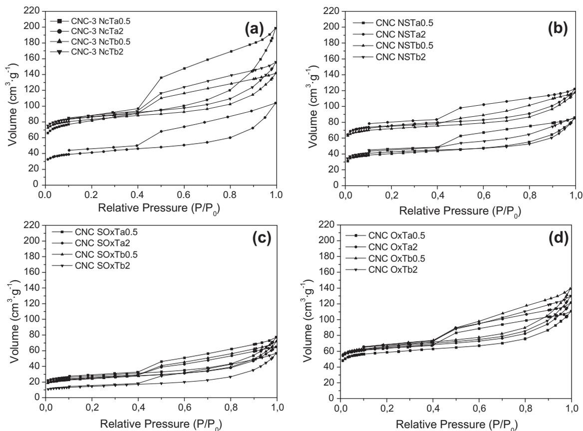
**Fig. 4.** Nitrogen adsorption-desorption isotherms of: (a) Samples treated with  $\text{HNO}_3$ ; (b) Samples treated with  $\text{HNO}_3\text{-H}_2\text{SO}_4$ ; (c) Samples treated with  $\text{H}_2\text{SO}_4\text{-H}_2\text{O}_2$ ; and (d) Samples treated with  $\text{H}_2\text{O}_2$ .
