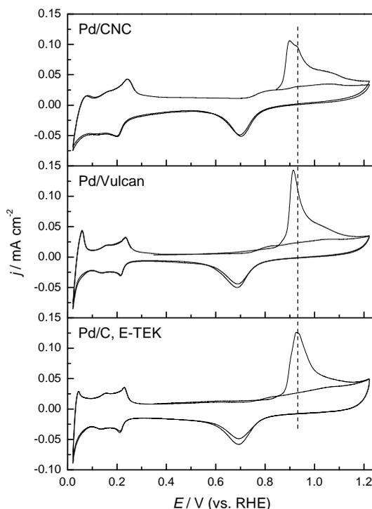
**Figure 4.13.** CO stripping voltammograms for the Pd/CNC, Pd/Vulcan and Pd/C from E-TEK electrocatalysts in 0.5 M H<sub>2</sub>SO<sub>4</sub>.  $E_{ad} = 0.056$  V;  $v = 0.020$  V s<sup>-1</sup>;  $T = 25$  °C.
