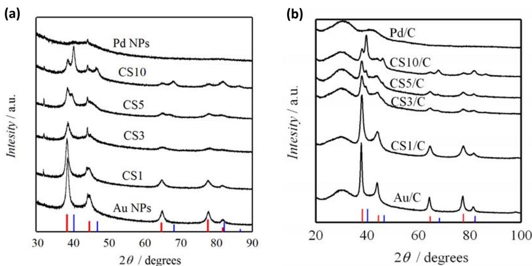
**Figure 4.27.** Powder XRD diffractograms of the various metallic nanostructures assembled on ITO (a) or supported on Vulcan (b). The red lines at the bottom of the graph, at  $38.1^\circ$ ,  $44.4^\circ$ ,  $64.6^\circ$ ,  $77.5^\circ$  and  $81.7^\circ$  indicate the standard Au diffraction pattern (PDF 040784), while the blue lines at  $40.1^\circ$ ,  $46.7^\circ$ ,  $68.1^\circ$ ,  $82.1^\circ$  and  $86.6^\circ$  belong to Pd (PDF 461043) [MONTES DE OCA 2012, CELORRIO 2012].
