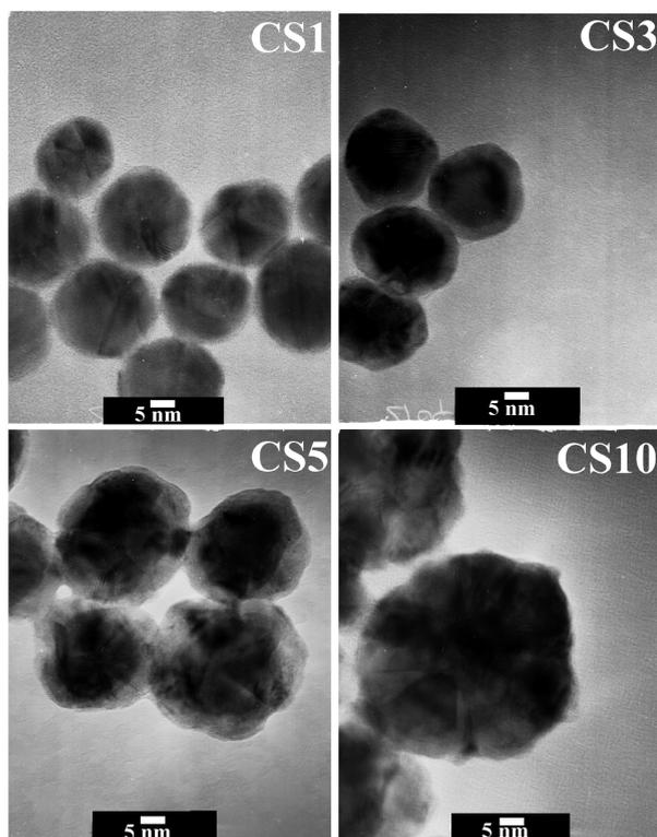
**Figure 1.** TEM images of Au–Pd nanoparticles featuring a  $19.3 \pm 1.2$  nm Au seed coated with Pd shells with thicknesses of  $1.3 \pm 0.1$  nm (CS1),  $2.7 \pm 1.0$  nm (CS3),  $5.1 \pm 0.9$  nm (CS5), and  $9.9 \pm 1.0$  nm (CS10).
