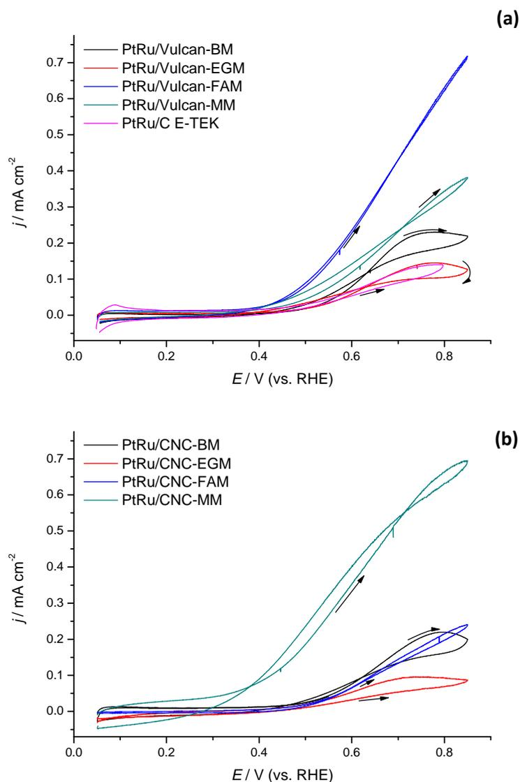
**Figure 4.15.** Cyclic voltammograms for the PtRu/Vulcan (a) and PtRu/CNC (b) electrocatalysts in 2 M  $\text{CH}_3\text{OH}$  + 0.5 M  $\text{H}_2\text{SO}_4$ ,  $v = 0.02 \text{ V s}^{-1}$ ;  $T = 25 \text{ }^\circ\text{C}$ .
