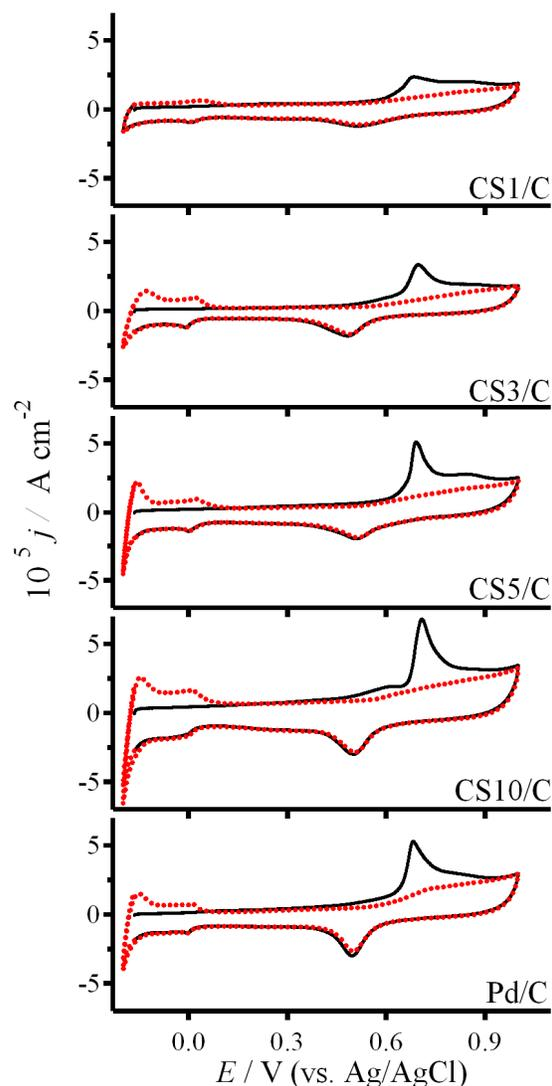
**Figure 4.** CO stripping voltammograms of the various nanostructures supported on Vulcan, in  $0.5 \text{ mol dm}^{-3} \text{ H}_2\text{SO}_4$  solution, at  $0.02 \text{ V s}^{-1}$ . The black full line corresponds to the first cycle, while the second cycle is displayed as a red dotted line.
