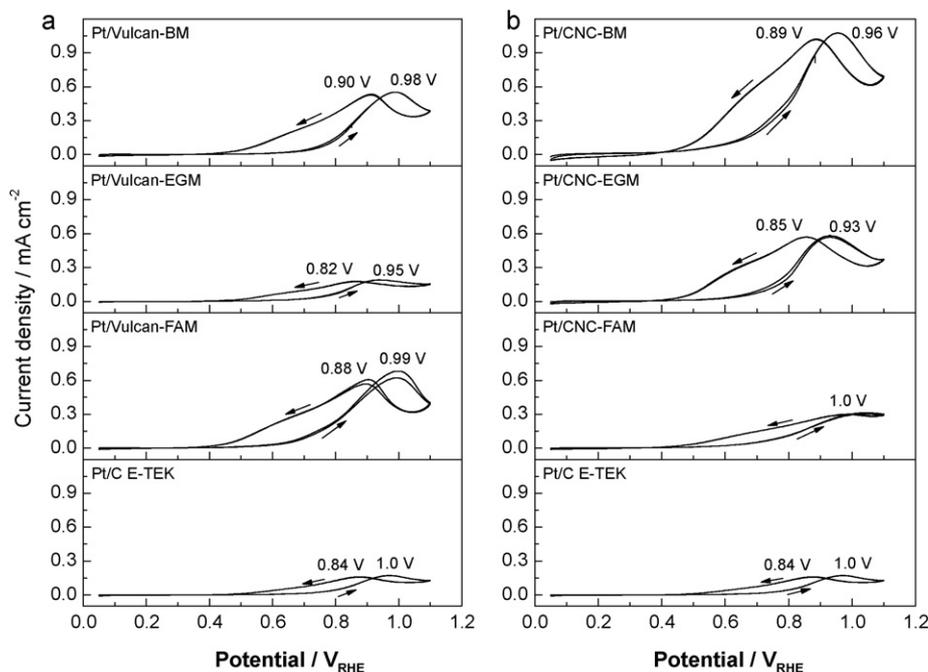
Fig. 3. Cyclic voltammograms for Pt/Vulcan (a) and Pt/CNC (b) electrocatalysts in 2 M  $\text{CH}_3\text{CH}_2\text{OH} + 0.5 \text{ M H}_2\text{SO}_4$ .  $\nu = 20 \text{ mV s}^{-1}$ ;  $T = 25^\circ\text{C}$ .
