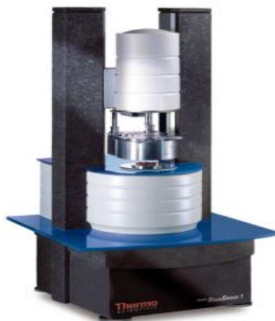
**Figura 9:** Reómetro HaakeRheoStress 1
