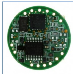
FIGURA 3.12 - Skyemodule M1-Mini ( http://www.digikey.com/ )
