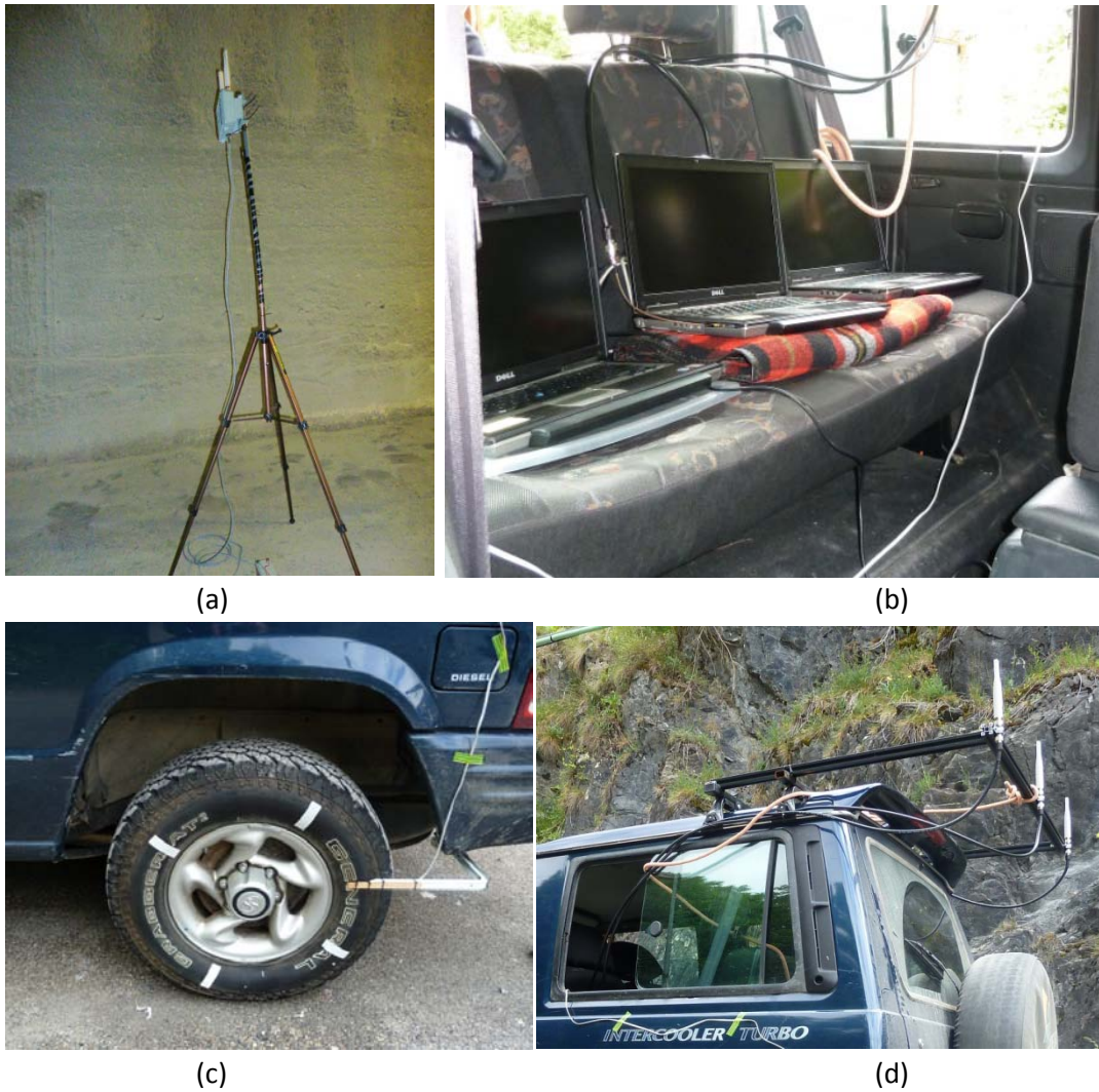
Figure 6. Large Scale Tool Modules: Communication module: Transmitter (a) and Receivers (b). Odometry module (c), and antenna platform (d)
