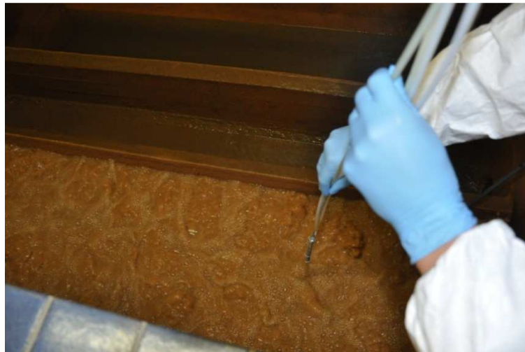
Fig.1.9 Placing the sampling tool
