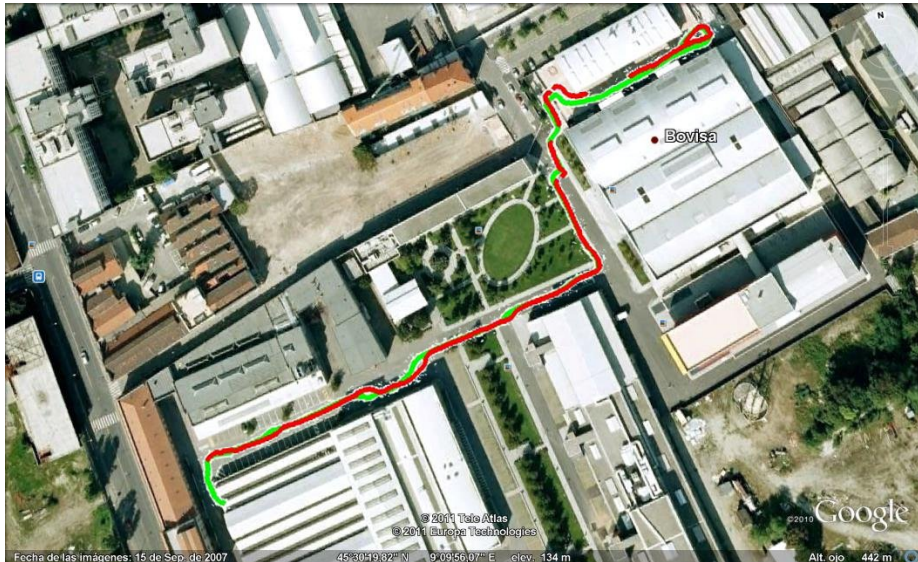
Figura E.10: GPS trajectory (red) and SLAM trajectory (green) superposed on the satellite image of the Campus of Bovisa (Milan) where the sequences were acquired
