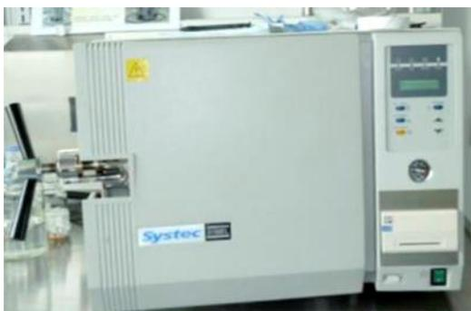
Fig. 3:6: Autoclave SysTec 3150 EL, FH OÖ, Campus Wels. Wels, Austria
