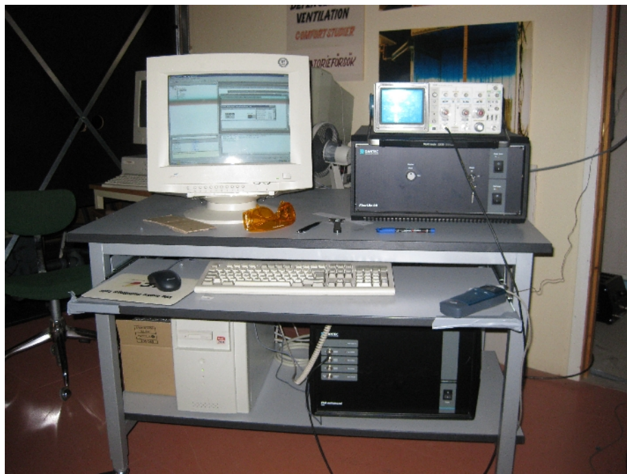
Figura 34. : Laser Doppler system; computer, laser optic system and electronic analyzer
