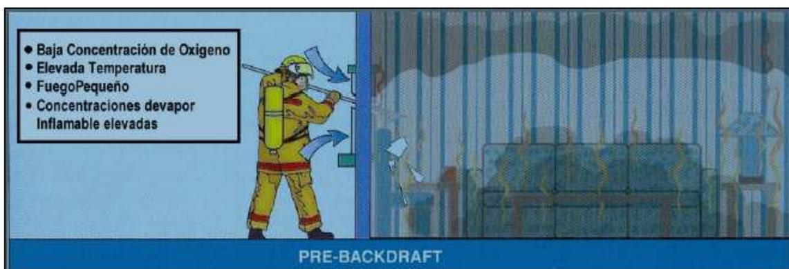
**Fig.23. Condiciones pre-backdraft.**
