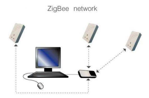
As we can see, there are some end-devices, which are the sensor modules, and a ZigBee coordinator module, in this case the datalogger module.
