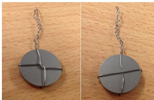
Figure 4.13 Front and back view of the wiring of the sample. The disk seen here is an unpolished tungsten sample.
