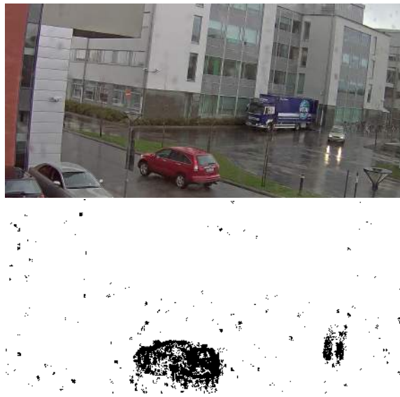
Figure 4.25: Showing the detection of the chromatic algorithm. The red moving car and the moving reflection of the headlights are detected while the stationary blue truck remains undetected.
