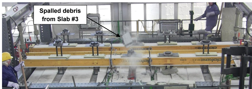
Fig. 1 – Testing Furnace, Explosive Spalling and Imminent Failure of Slab #3 at 22' 10''.
