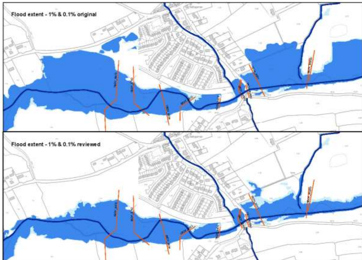
Figure 2 Example flood mapping problem: (upper) incorrect post-processing due to a user incorrectly applying GIS analysis to determine the water surface predicted by a 1D hydraulic model by intersection with a digital terrain model; and (lower) corrected post-processing when the user excluded the overlaying of water levels from tributaries on the primary river floodwater surface elevations. The problem was not straightforward to identify due to a lack of validation data.
