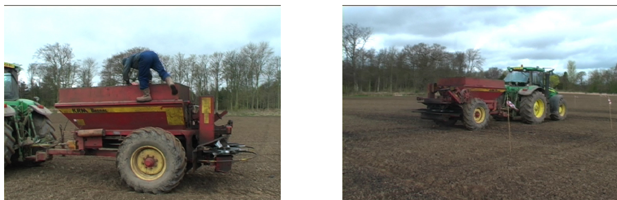
Figure 5.1: Spreading charcoal fines using a fertiliser spreader
