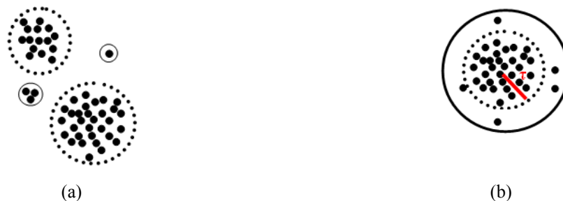
Fig. 1: (a) A representation of clustered data, for small clusters boundaries are shown with thick lines and dense clusters' boundaries are shown with dashed lines, (b) Outlier detection in dense clusters: samples which are inside of the inner circle are classified as the majority class whereas the rest of the samples are classified as the minority class, given threshold \tau .
