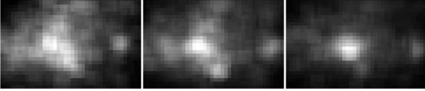
Figure 5. Voting spaces for three neighbouring viewpoints. Note how strong hypotheses appear at similar locations.
