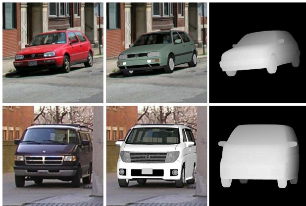
Figure 4. Obtaining depth maps for the car images. Left shows the original image, middle the image with the most suitable 3D model superimposed (notice how the model for the second car is a completely different brand, but still fits fairly well). The rightmost images show the depth maps obtained from the 3D model.
