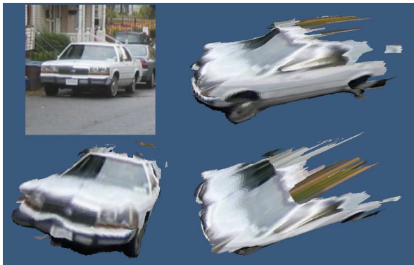
Figure 17: Some views of a texture mapped 3D model, generated from the depth map of the recognized car in the top left corner.
