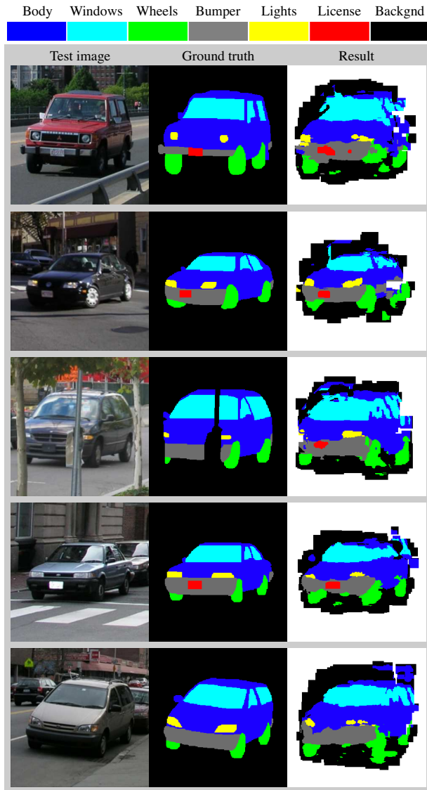
Figure 14: Results for the car parts annotation experiment. From left to right: test image, ground-truth, and output of our system. White areas are unlabeled and can be considered background.
