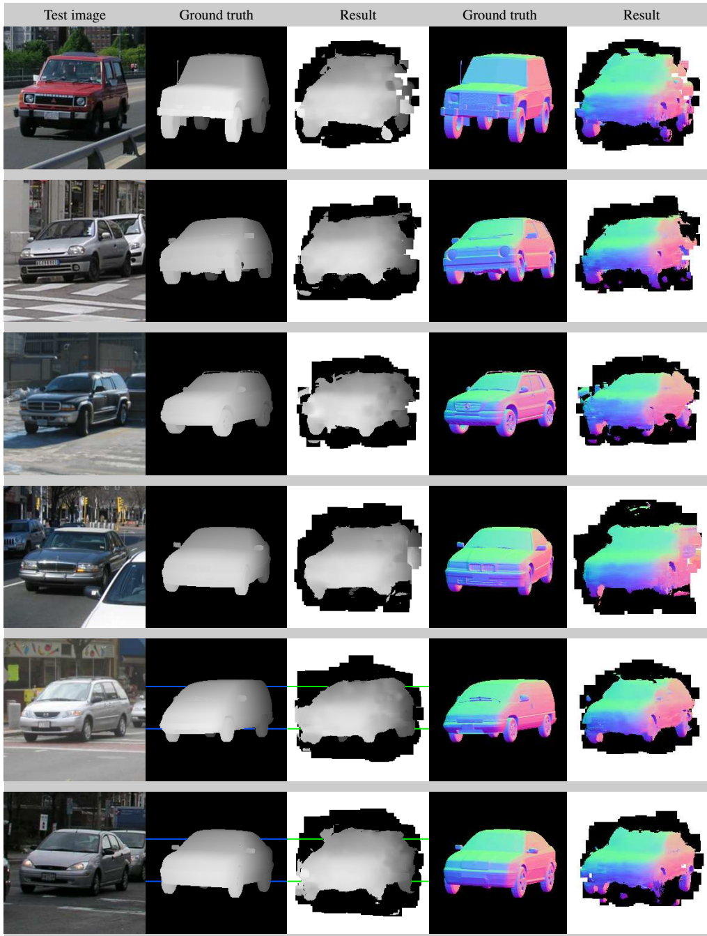
Figure 15: Results for the car depth map and surface orientation experiments. From left to right: test image, ground-truth and output of our system for the depth map experiment, and ground-truth and output for the surface orientation experiment. The R,G,B colors represent the components of the surface normal according to Eq. 13. White areas are unlabeled and can be considered background. The lines in the last two rows indicate the slices from Figure 16.
