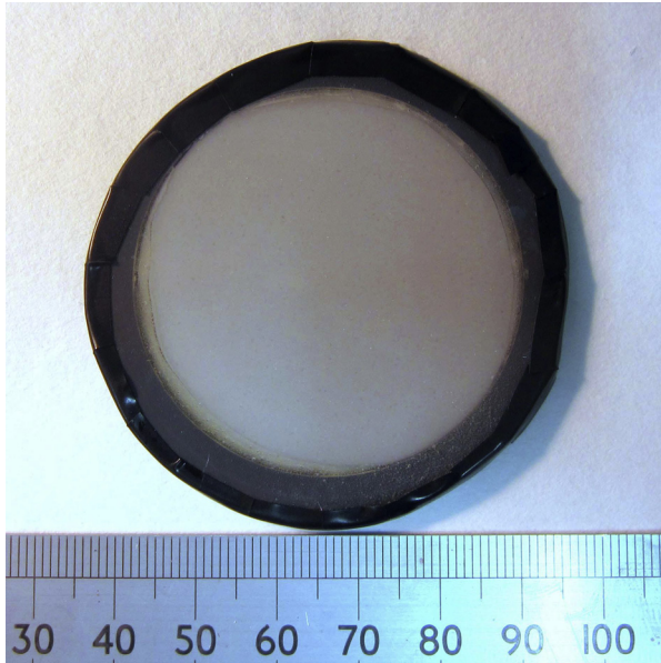
Fig. 1. Example konjac–carrageenan tissue-mimicking test cell.
